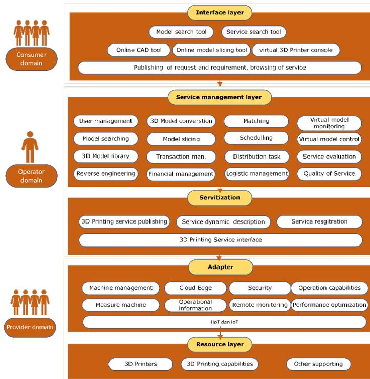
Figure 4. Cloud additive manufacturing architecture
